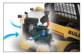
Efficient **KUBOTA** engine cooling with direct-mounted fan and cooler reduces fuel consumption.
